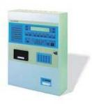
The ZP3 analogue addressable control panel range, in one, two and four loop versions, with peer-to-peer networking, allows for systems of up to 100 panels with over 50,000 sensors.
